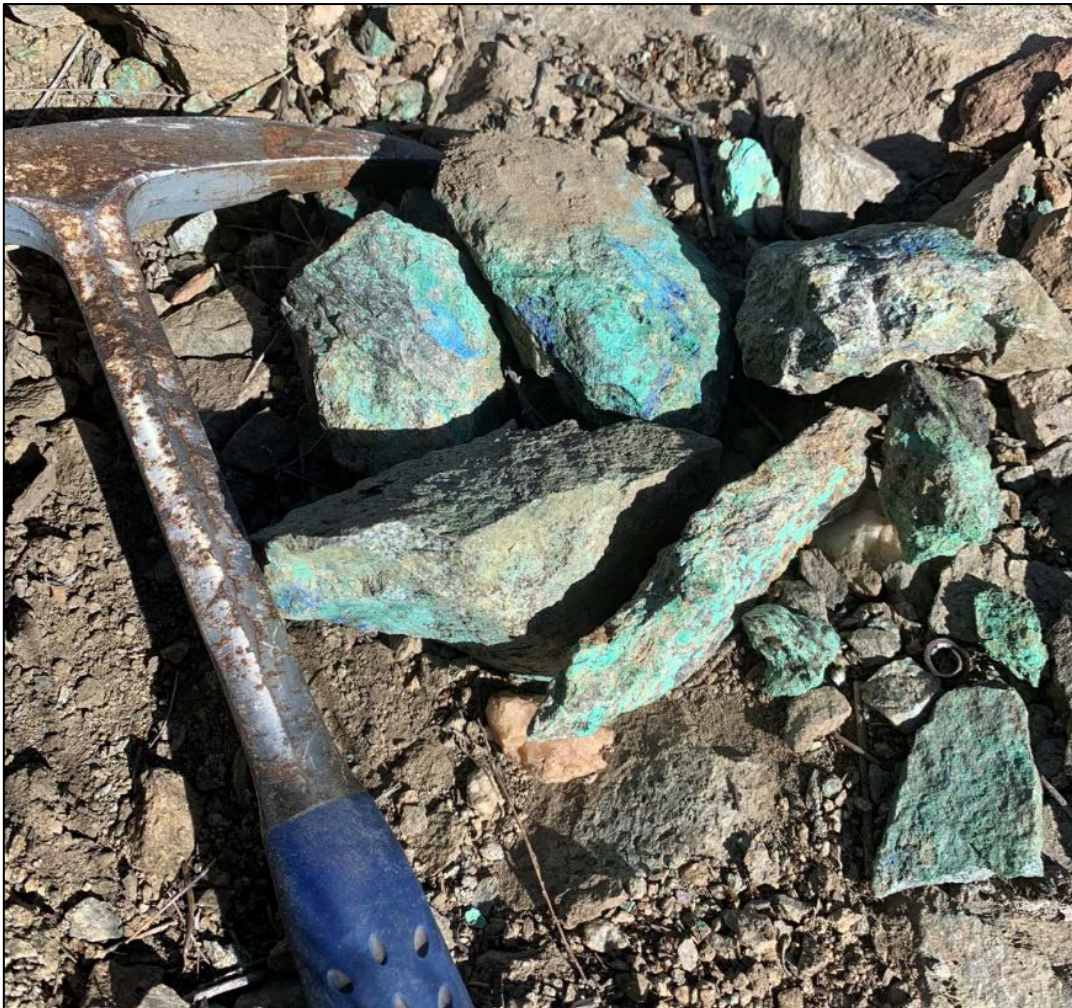
Figure 2 High-grade waste from dump material at OREX target assaying 9.15% Cu, 192 g/t Ag and 0.15 g/t Au. The sample was collected next to a small adit mined along a copper-bearing shear within the Leatherwood intrusive.
