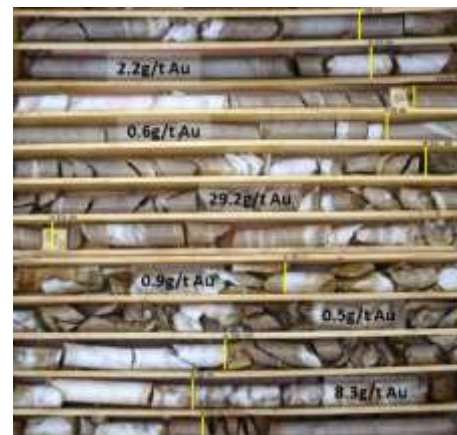
Figure 3: Core from DDH-02, 48-58m depth averaging 4.3g/t Au
