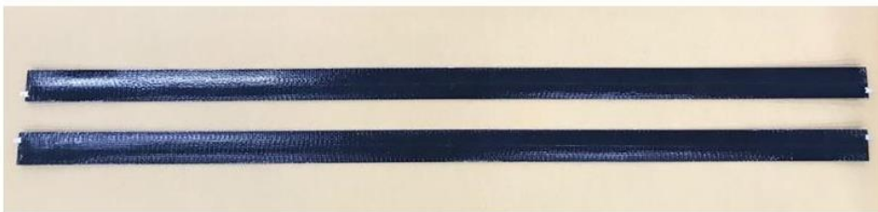
Test strip PV modules prepared by BeyondPV for Clearvue.
