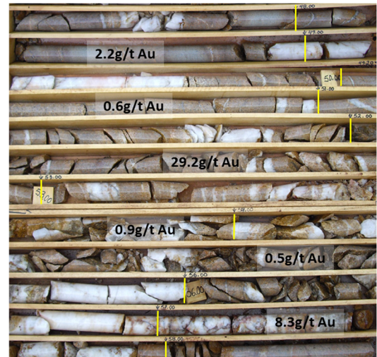
Figure 5: Core from DDH-02, 48-58m depth averaging 4.3g/t Au
