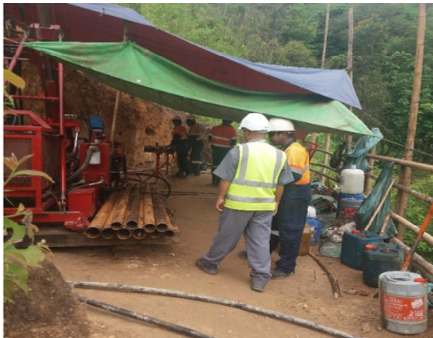
Figure 1. Man-portable rig drilling on Yegon Ridge.
