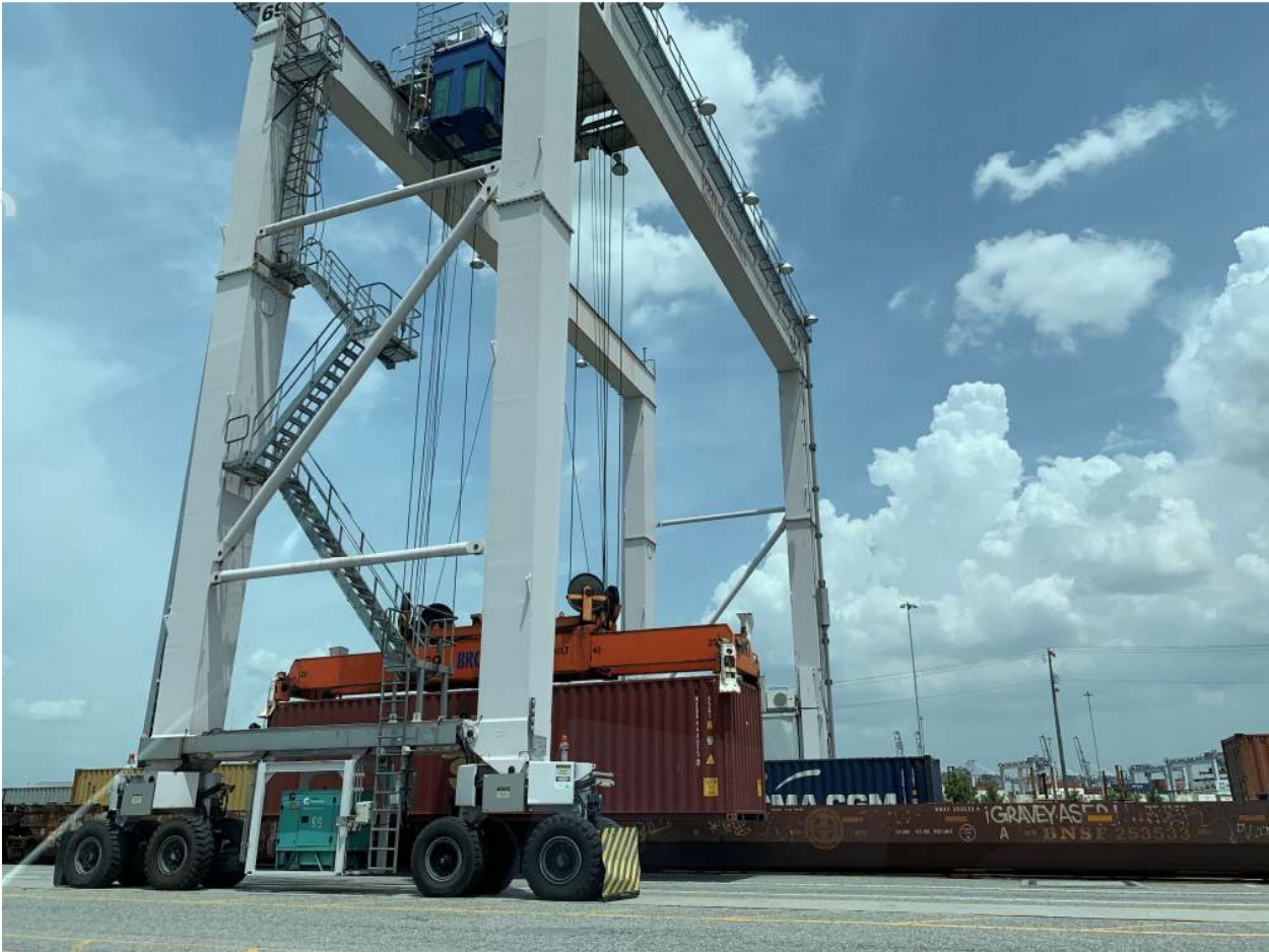
Figure 4. One of approximately 150 rubber tyred gantry cranes currently operating at Port of Savannah
