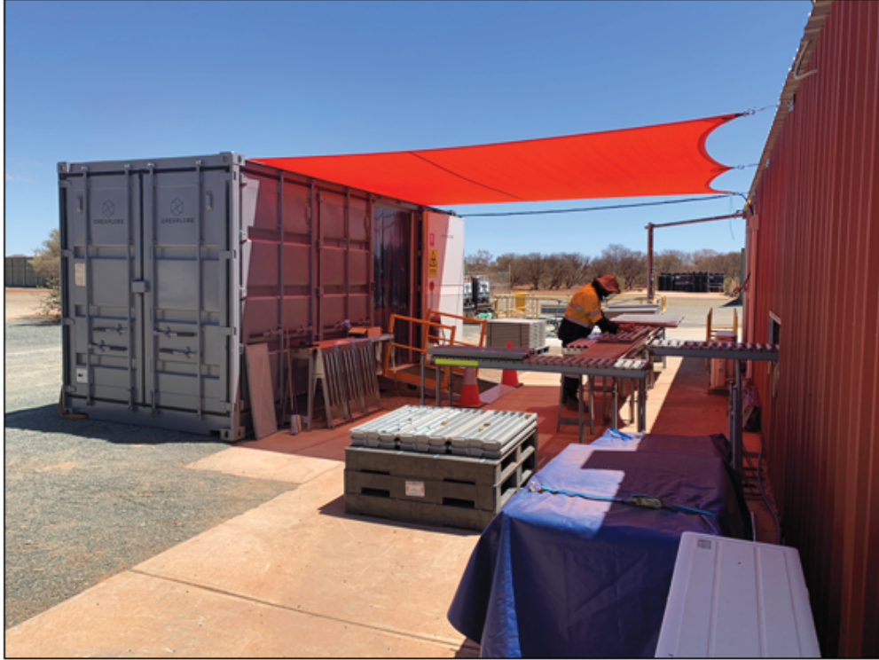
Fig 1. Orexplore site-based laboratory housing three GeoCore X10 machines established next to client's core farm and scanning core.
