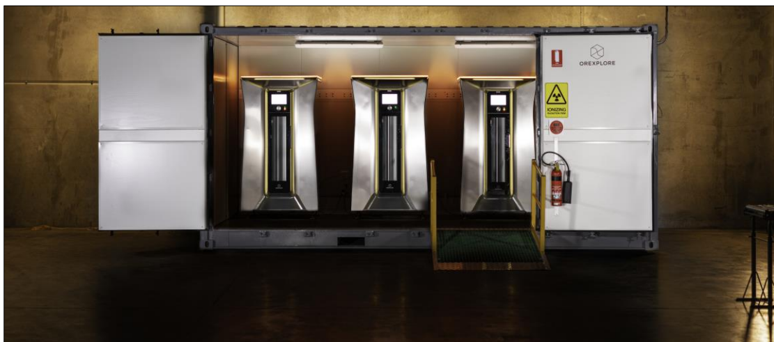
Fig 2. Oreplore field container with three GeoCore X10 instruments capable of scanning over 5,000m of core per month generating unique 3D tomographic imaging, through the core geochemistry and a host of other automated outputs.
