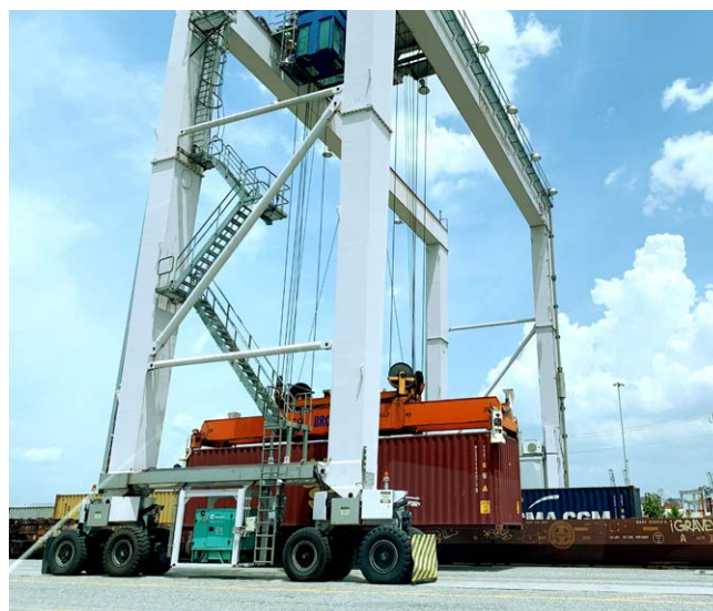
Figure 2. Container crane at Port of Savannah showing wheels on "runway"
