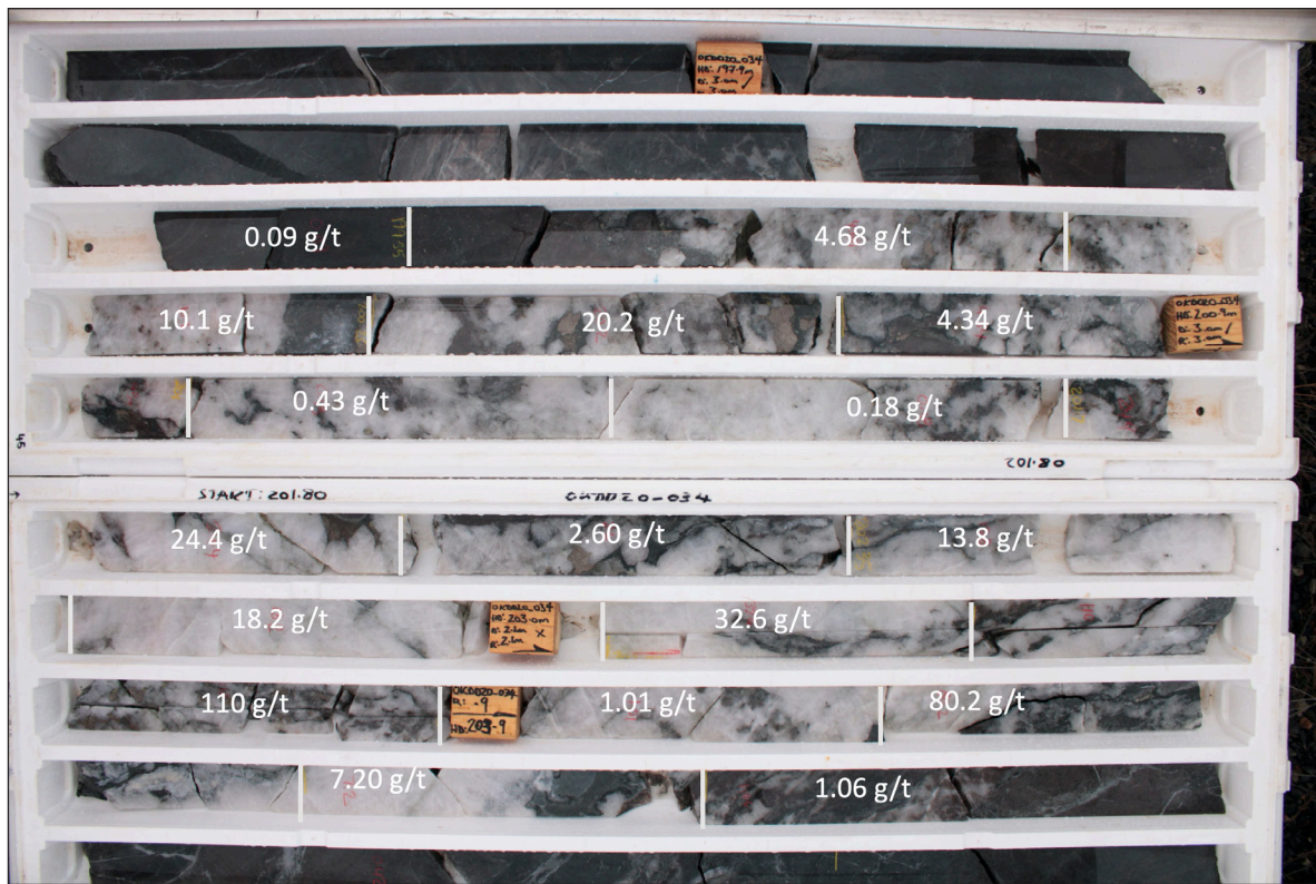
Figure 3: High grade gold intersection from the O2 Lode - 6.05 m @ 22.9 g/t from hole OKDD20_34
