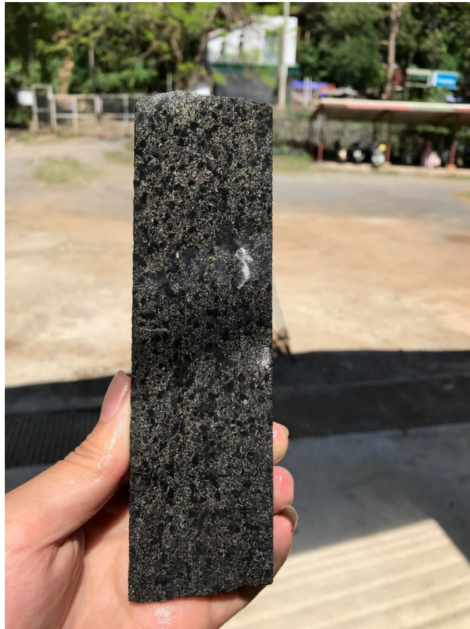
Figure 3: Blackstone's Ban Chang drillhole BC20-04: net-textured Ni and Cu sulfides in ultramafic rock
