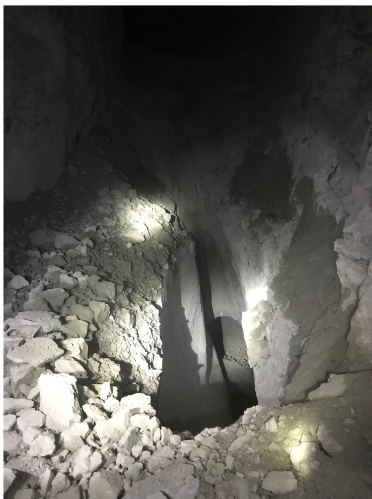
Avoca stope prior to backfill being placed
