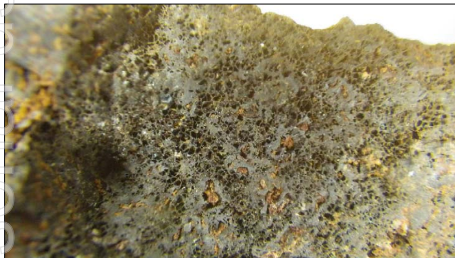
Figure 6 Goethitic gossan rock sample – field of view approximately 3 cm.
