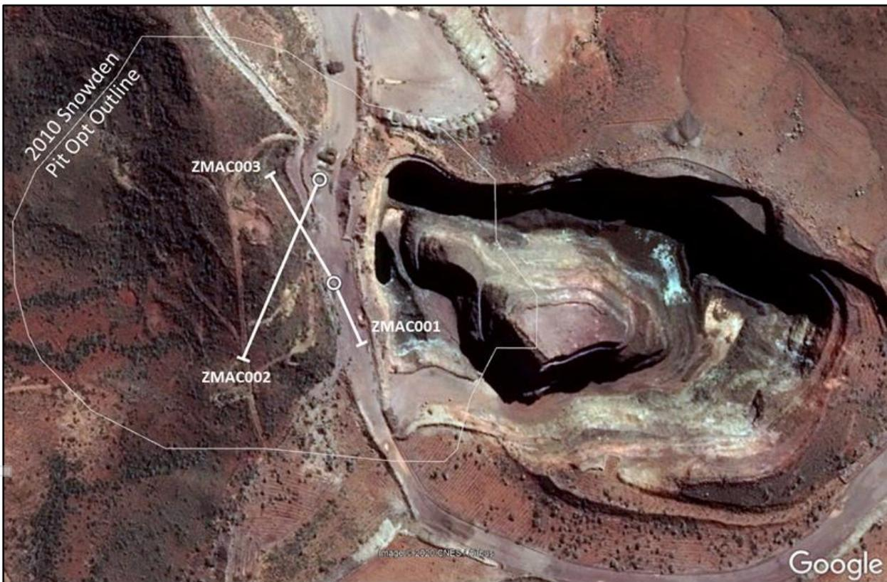
**Figure 6: Proposed Metallurgical Resource Drilling adjacent to Mons Cupri Pit**
