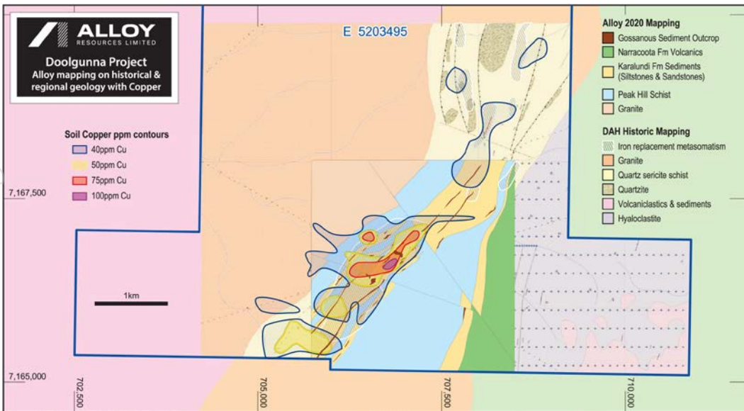
Figure 4 Company geological mapping over Peak Resources 2010 map and showing Cu soil anomaly.
