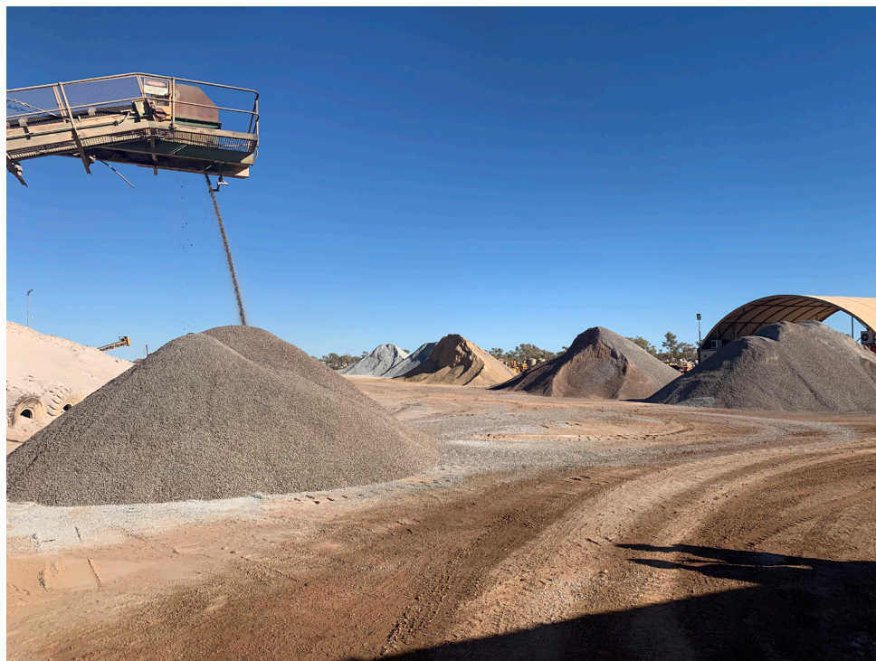
Crushed ore stockpiles ready for milling at Halls Creek
