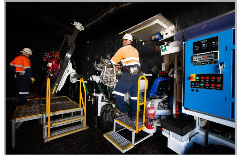
DeepEX prototype drill in use – capable of >2,000m diamond core holes from underground.
