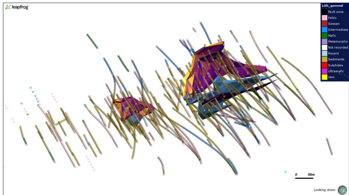
Figure 5-2: Plan view of DD and RC drilling and the interpreted domains for Salt Creek prospect
