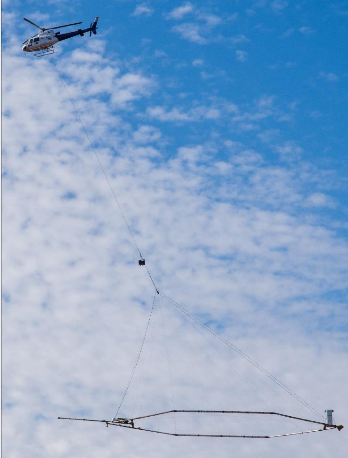
Figure 3: SkyTEM helicopter-borne electromagnetic surveying equipment in flight at Strickland
