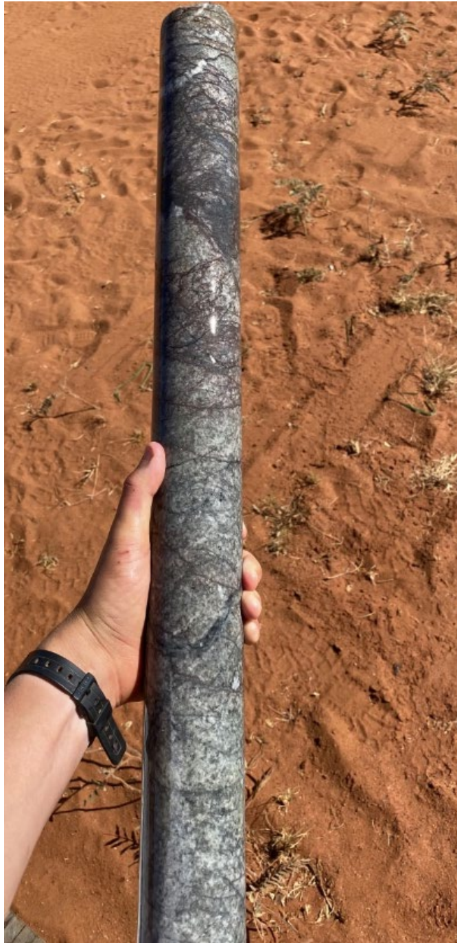
Figure 6 Falcon HERC236D – Close up of intense brecciation and alteration.
