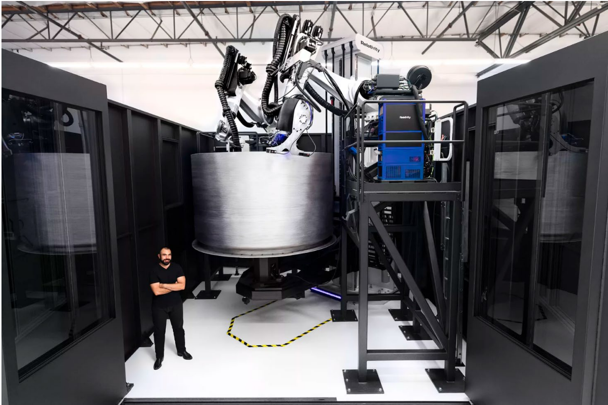
3D printing of the Terran 1 launch vehicle at Relativity's Stargate factory
