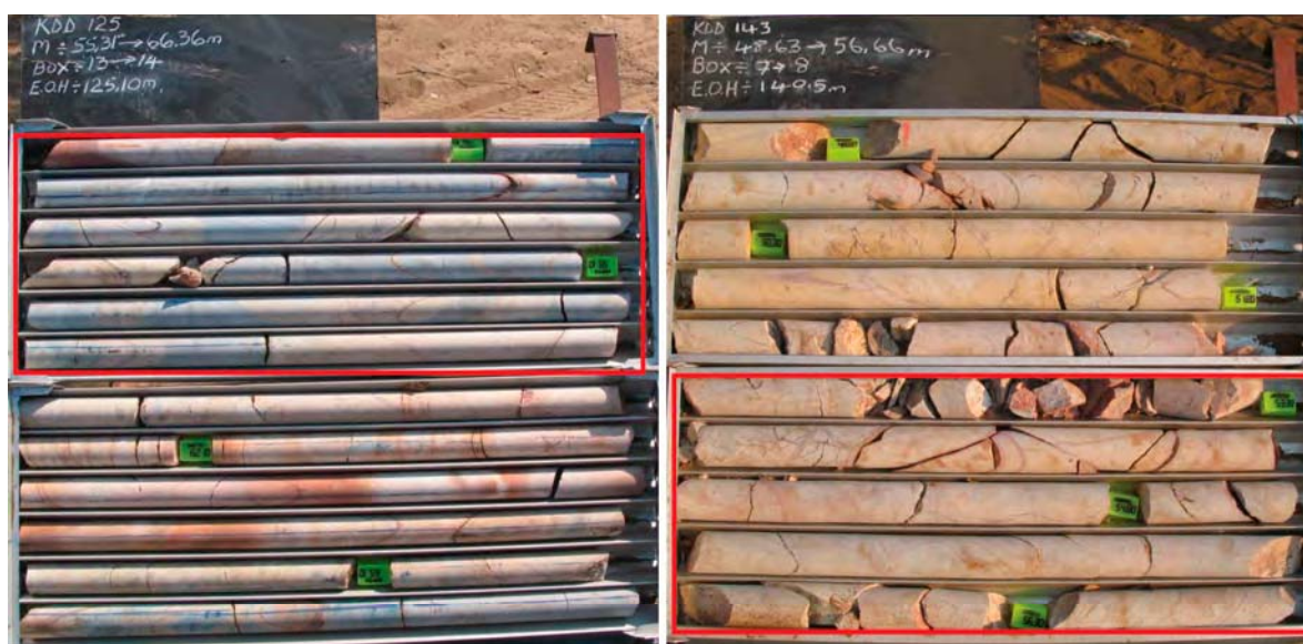
Figure 5. Pictures of drillcore trays with the analyzed drillcore intervals (enclosed in the red line): KDD 125: interval 55.00–60.90; and KDD 143: interval 50.00–54.93. In both the cores it is possible to see reddish intervals, affected by supergene alteration.
