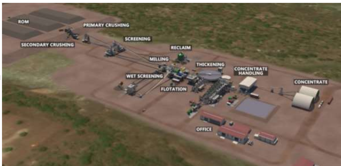
Figure 5: Rendered View of the Process Plant
