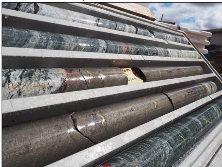
Photo 1 – Nickeliferous (Po-Pn-Cpy) massive sulphides intersected in SNDD0013 at the Saint Andrews Target of the Saints Nickel Project
