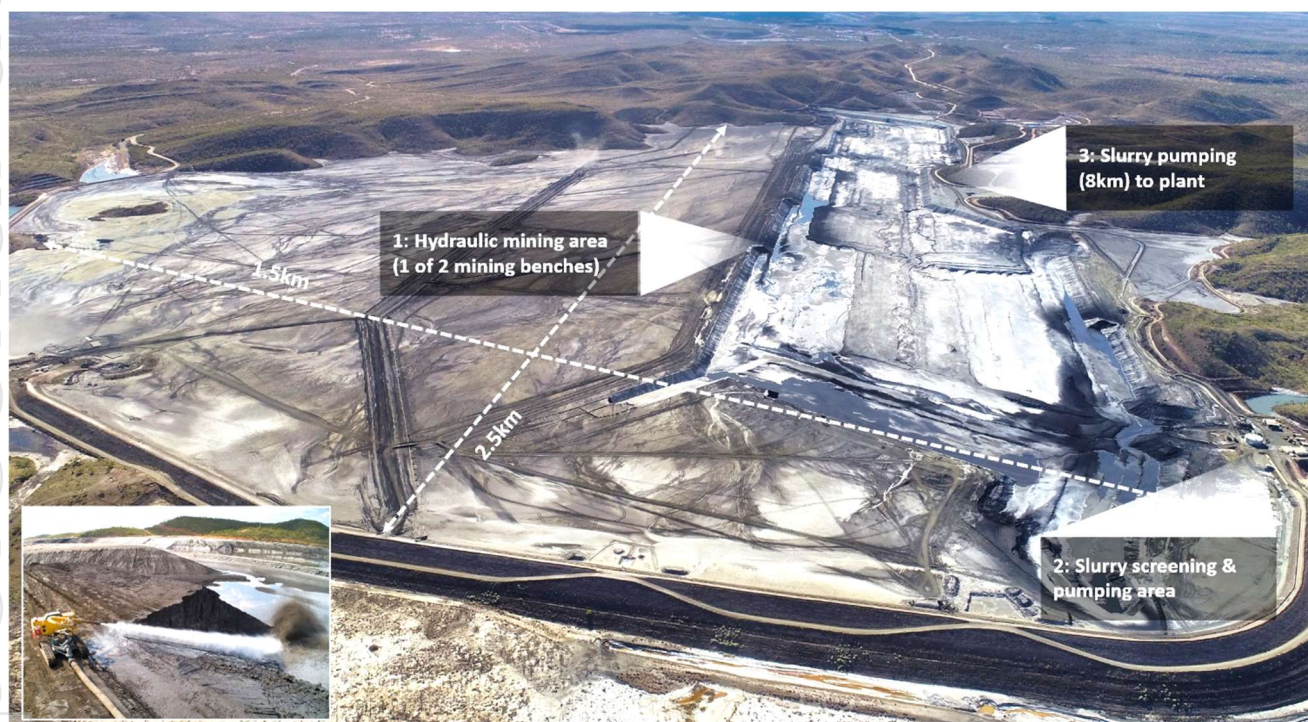
Figure 6: Overview of hydraulic mining operations at Century
