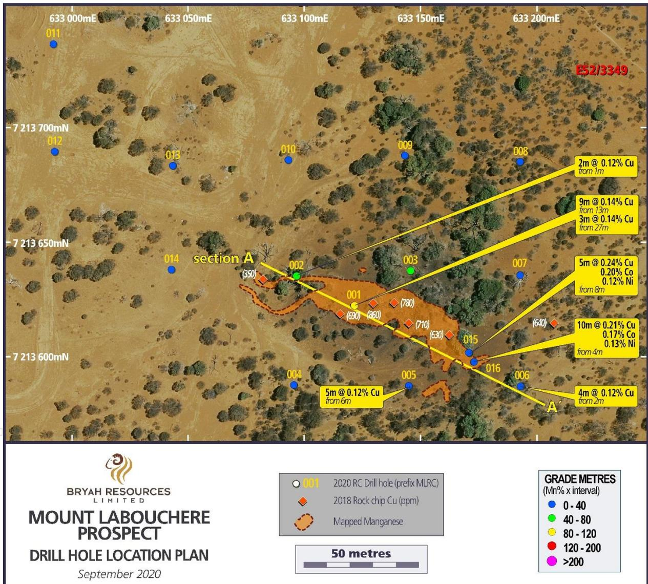
Figure 5 – Mount Labouchere Prospect - Drill Hole Location Plan
