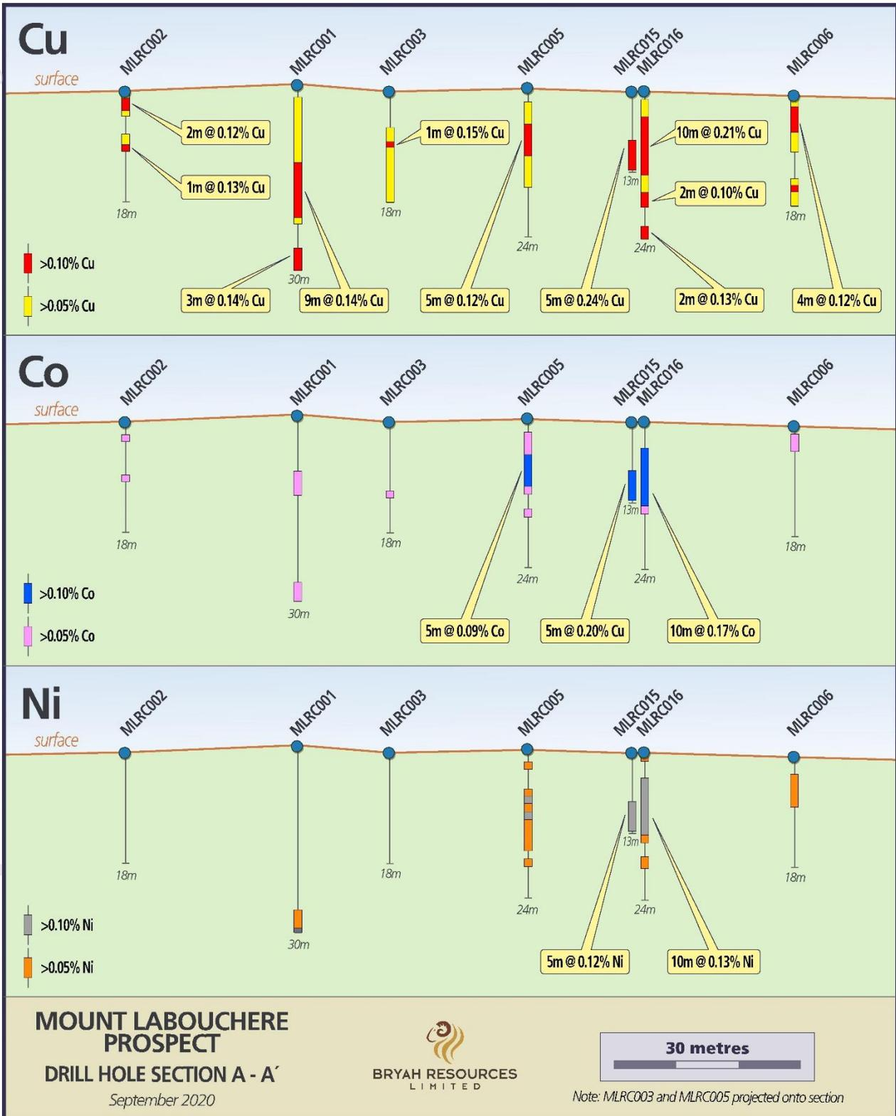
Figure 6 - Mount Labouchere Prospect Drill Hole Section A-A'
