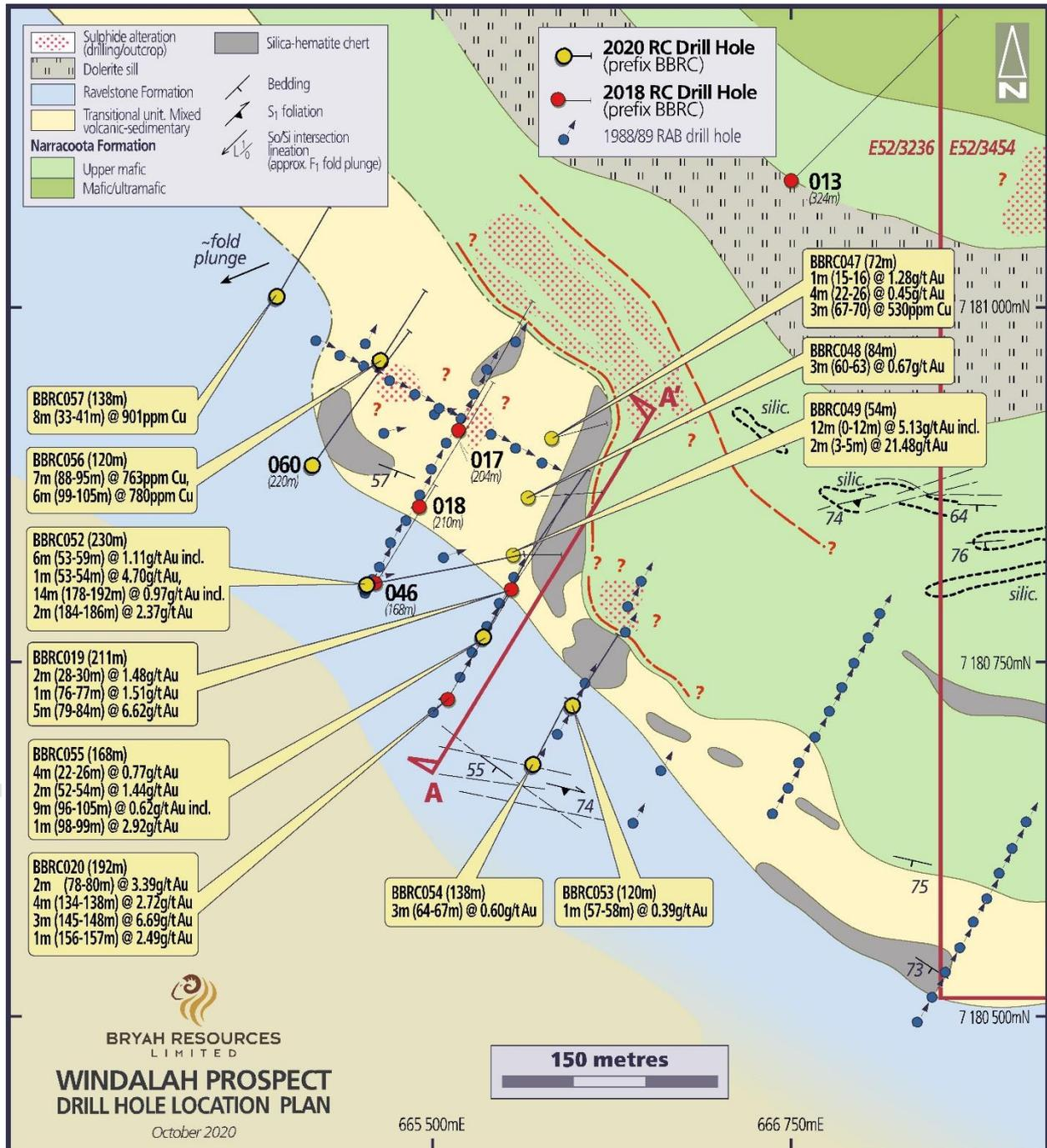
Figure 2 – Winalah Prospect Drill Hole Location Plan
