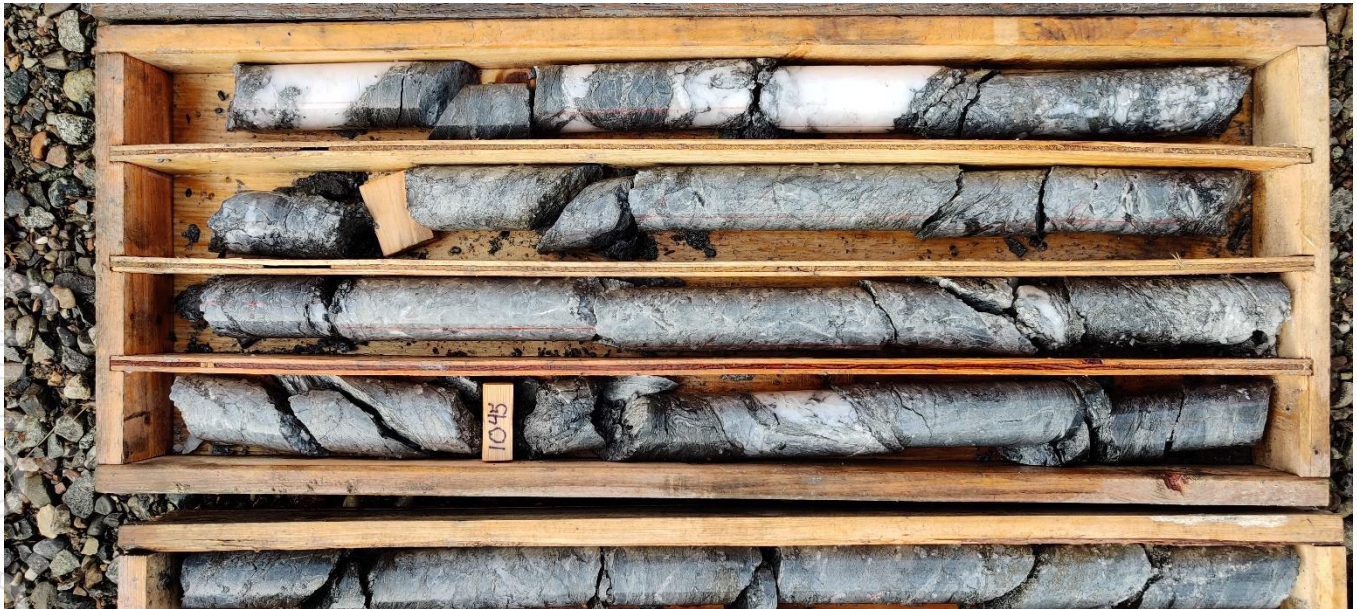
Figure 7: Drill core from the zone of silicification, quartz veining and brecciation in LC20-06 at Sidewinder Blowout.
