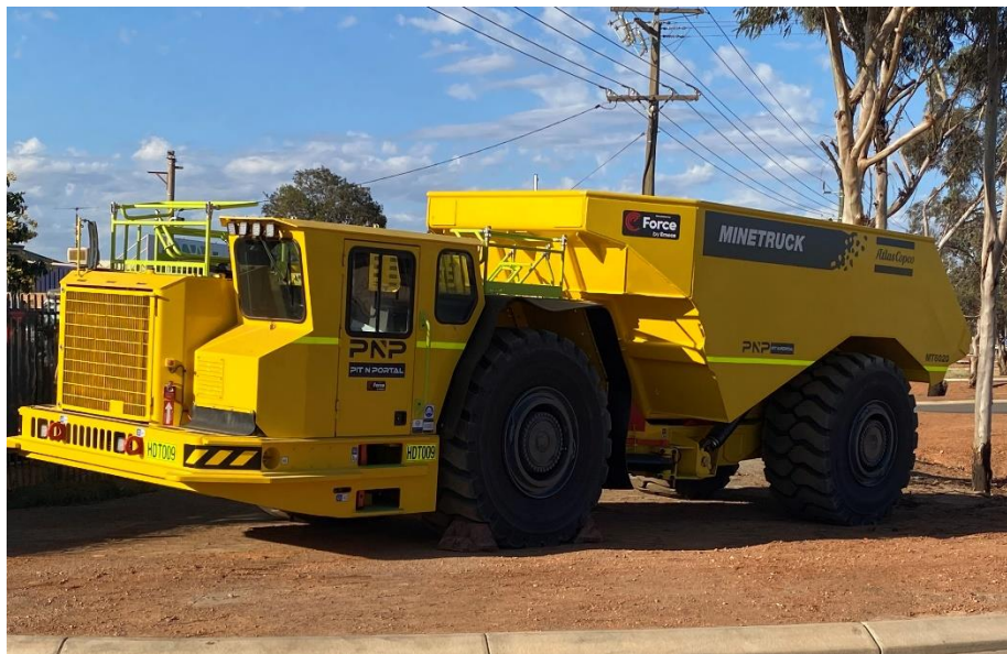
Fully refurbished 60-tonne underground haulage truck for Cassini
