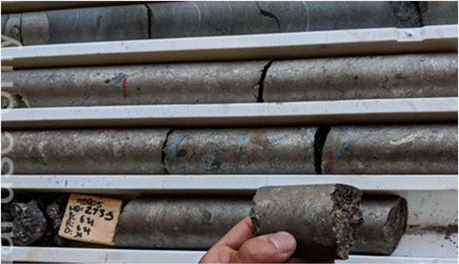
Figure 14 | Massive Sulfides in TOR05 from drilling at the Thor Prospect
