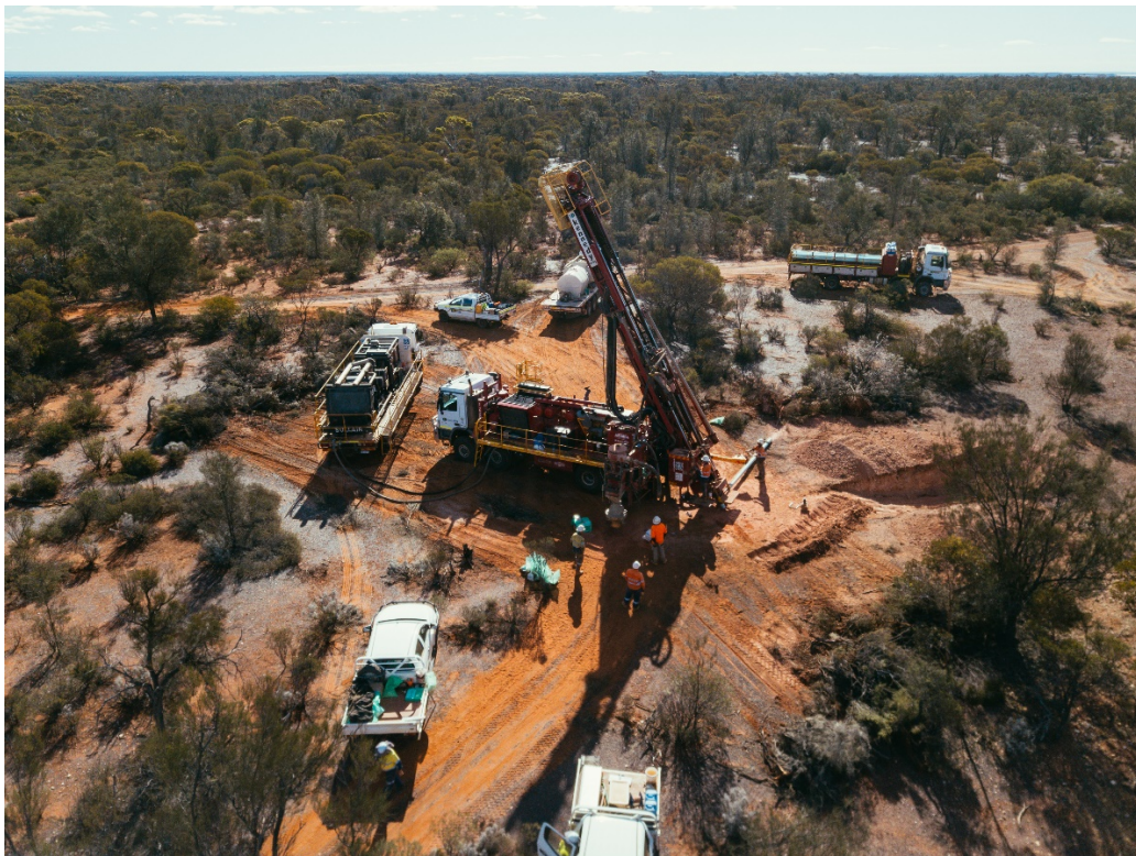
Figure 7: RC drilling in progress at the Grafter, Lady Charlotte target.
