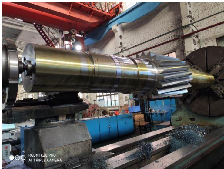
Ball mill head and pinion manufacture
