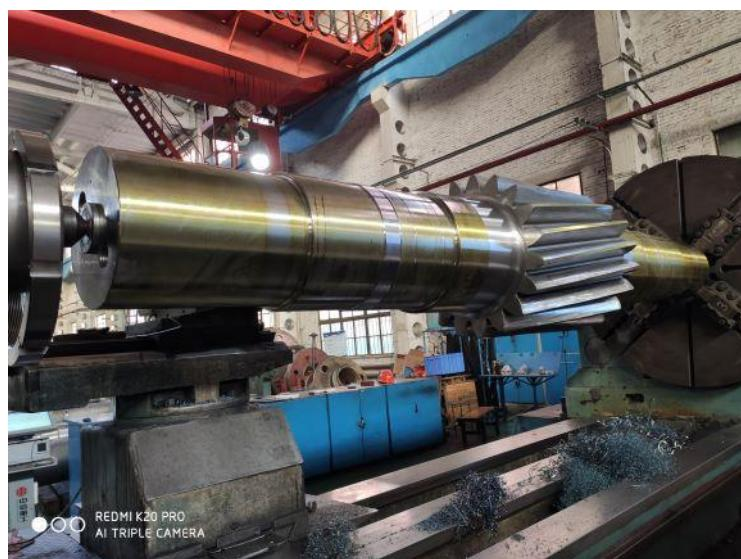
*Ball mill head and pinion manufacture*
