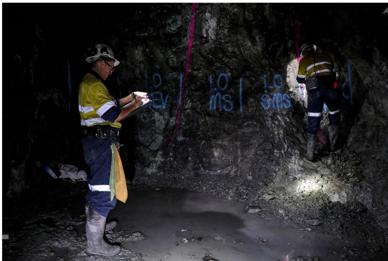
Figure 1 Mapping and sampling an ore drive face in Far West
