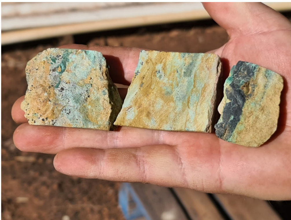
Figure 4: drill core showing the cross-cutting nature of the copper mineralisation
