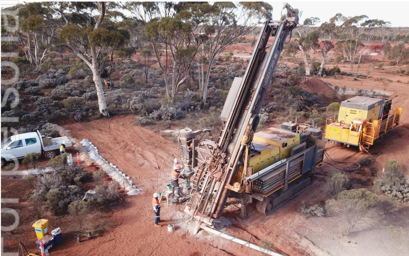
Image 4 – RC drill rig at Mandilla East
