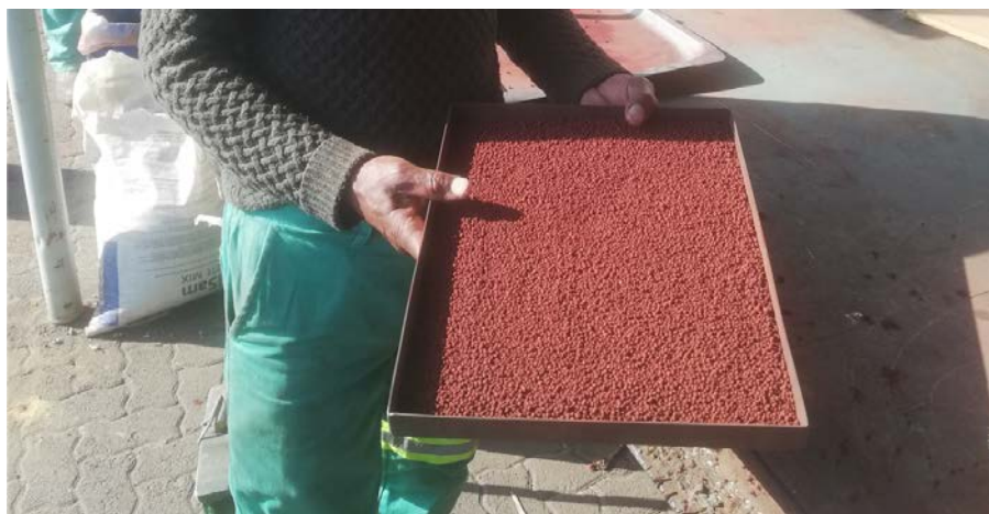
Figure 3: Agglomeration of iron fines into pellets
