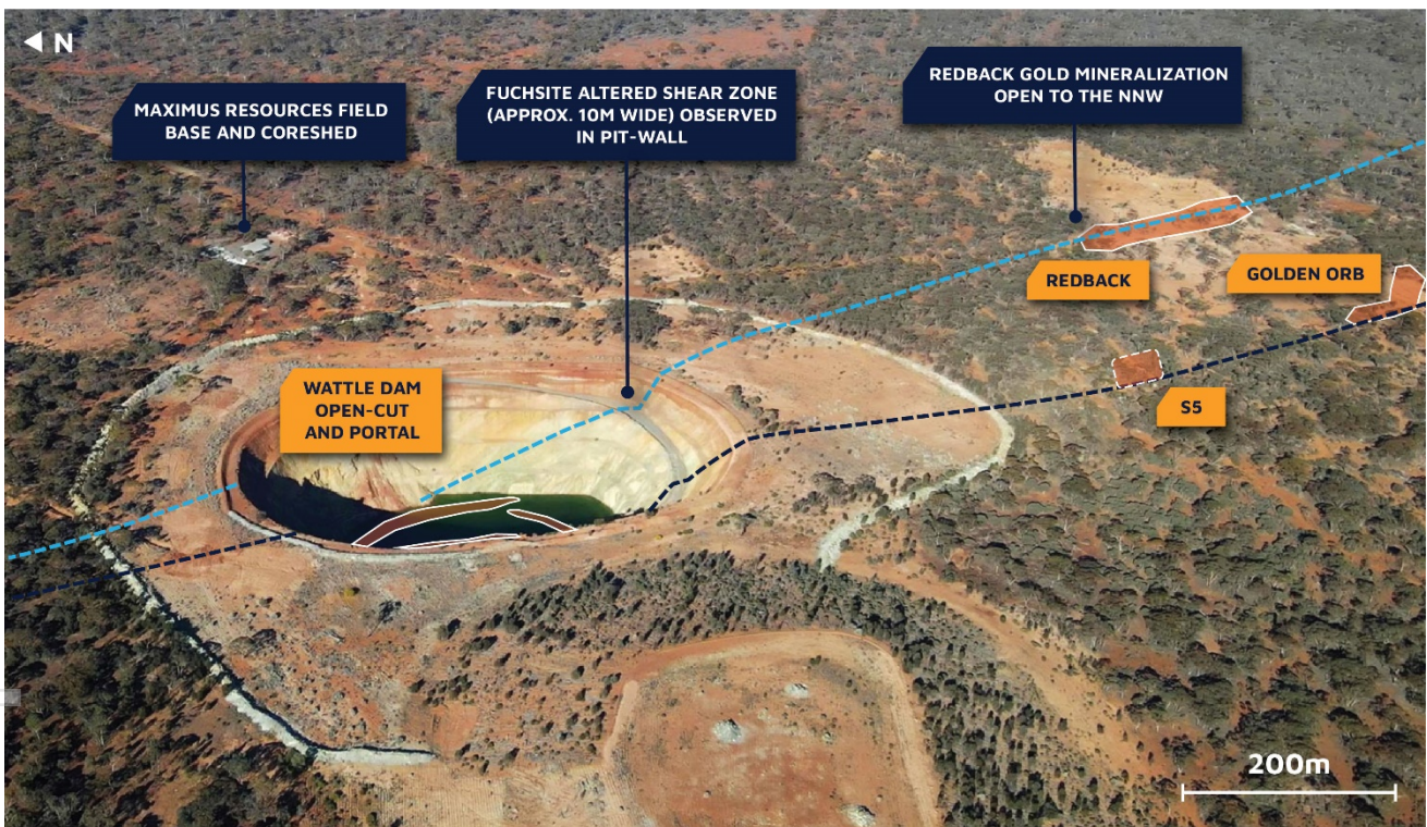
Figure 1. View looking East: Wattle Dam Gold Mine and Maximus prospects to the SSW. Dashed lines represent interpreted shear zones. Note that the actual geometry of the S5 prospect requires drilling to improve understanding and this is the focus of the upcoming RC drilling programme. The representation of mineralisation in the Wattle Dam Open-cut is now mined-out.
