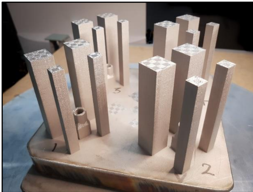
Fig 1: Tensile Bars printed at high laser power
