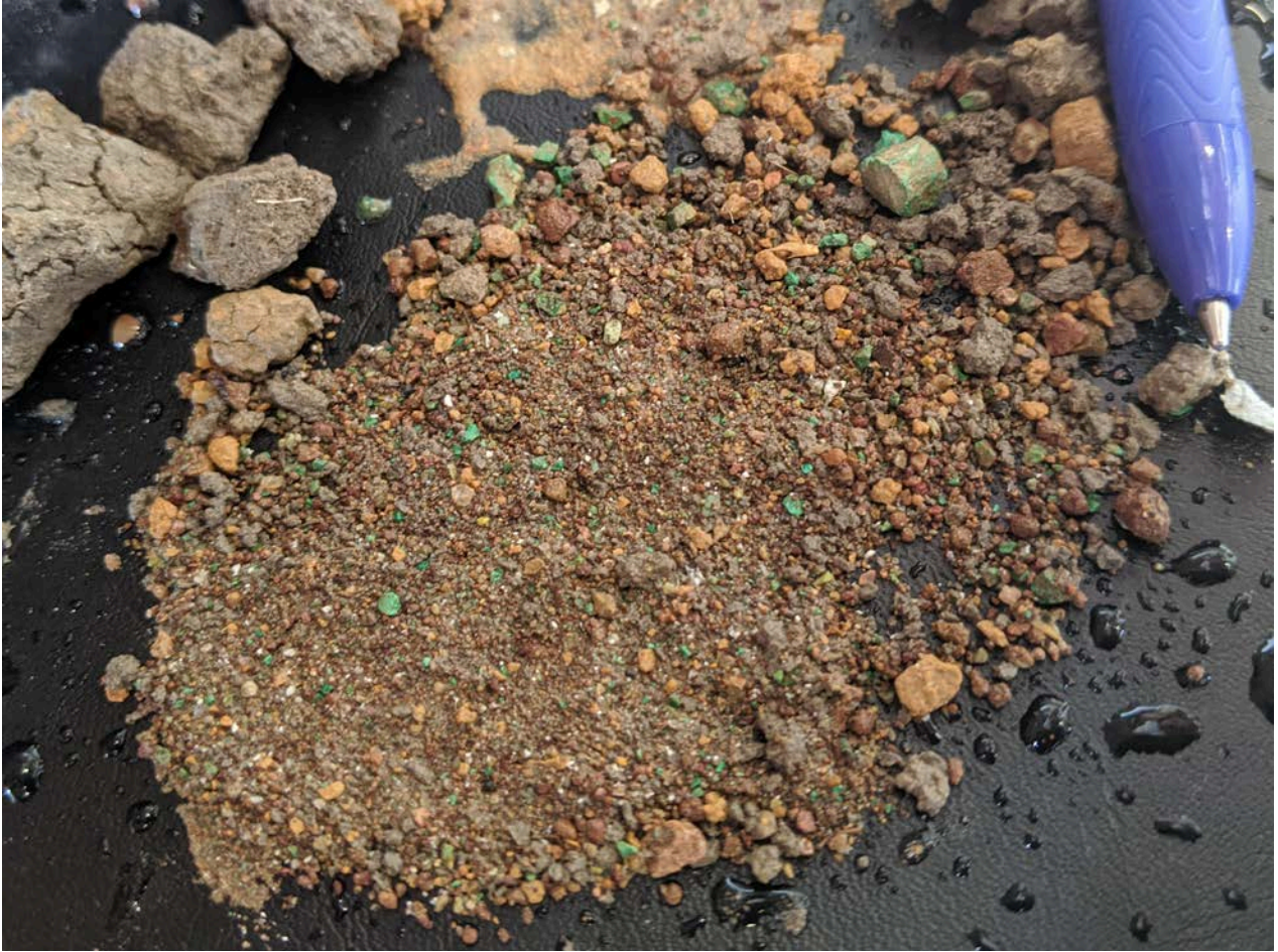
Photo 5 – Copper Carbonate (Malachite) mineralisation at Jessica: 0-3m from RN28419 – chemical assay 1.5% Cu
