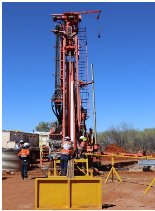
Figure 1: Setting the collar pipe for 20CRD001 at Rover 1, August 2020
