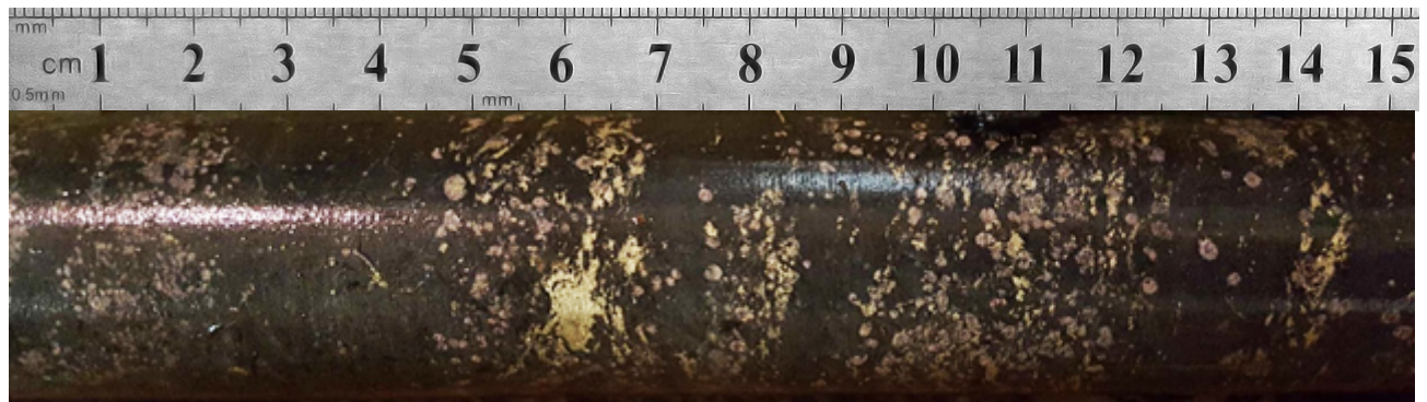
Figure 5: Photo of 36mm diameter Diamond Drill Core - Mineralisation style encountered in drill hole GRO20-02 at Green Mile. Biotite-Garnet-Amphibole alteration with 1-5% including visual chalcocopyrite and minor pyrite, at 33.1m metres down.
