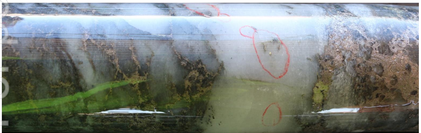
Figure 9: DRDD521 444.6m-445.5m Smokey grey quartz veining with moderate pyrrhotite and chalcopyrite fracture fill in addition to trace arsenopyrite. Vein has 20+ flecks of visible gold, largely associated with a hairline fracture through the full thickness of the vein. Assays pending
