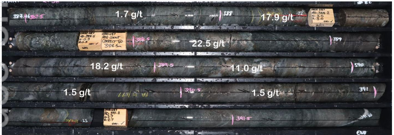
Figure 4: Deacon Central extensional DRDD487, smokey quartz associated with biotite amphibole shearing, 20% pyrrhotite and trace chalcopyrite. Interval assayed 3.5m @ 10.5 g/t gold. The intercept is located in the Deacon Central area with the nearest drill holes >200m in every direction. The mineralisation is the shallowest significant intercept to date from Deacon, and may represent the up plunge extent of Deacon Main.
