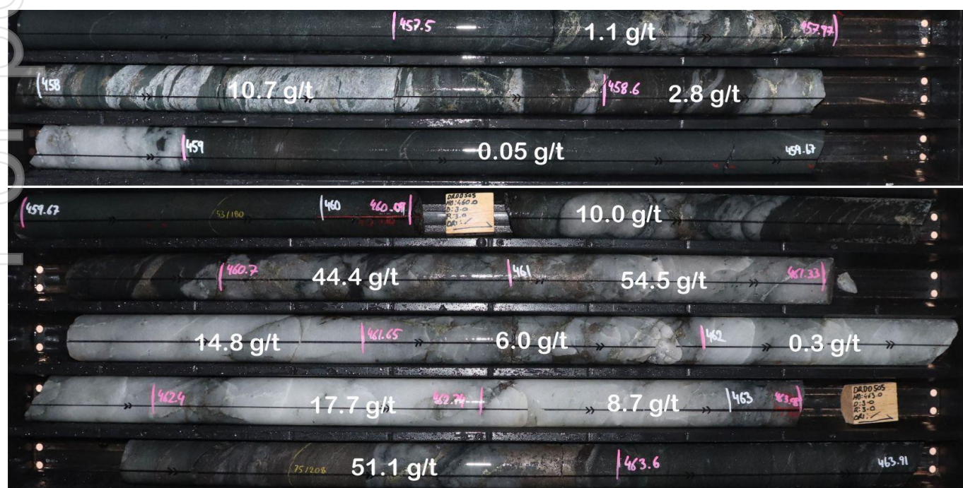
Figure 6: Bellevue North Lode extensional DRDD505. Milky and smokey quartz associated with biotite amphibole shearing, 10% pyrrhotite and trace chalcopyrite. +10 flecks of visible gold observed. Interval assayed 6.1m @ 14.5 g/t gold. The intercept is located in an untested area of the Bellevue lode below the deepest historical level development.
