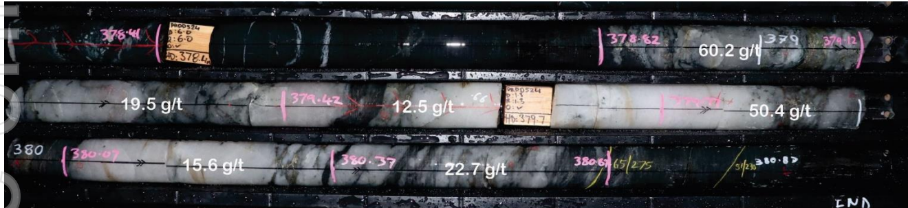
Figure 11: DRDD513 Milky quartz veining with narrow zones of smokey grey quartz. Equal amounts of pyrrhotite and chalcopyrite fracture fill. 20+ flecks of visible gold. Interval assayed 1.9m @ 58.0 g/t gold
