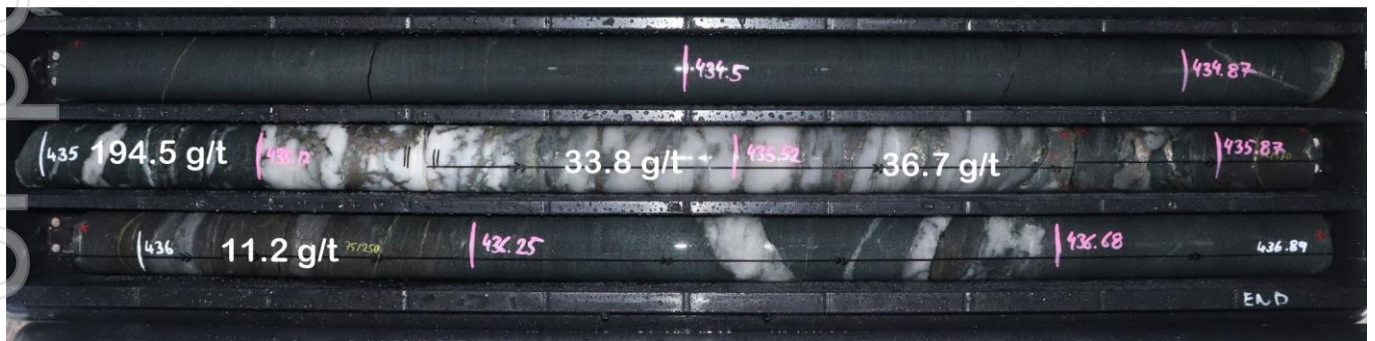
Figure 3: Deacon North extensional DRDD495. Milky quartz associated with biotite amphibole shearing, 10% pyrrhotite and trace chalcopyrite. +12 flecks of visible gold observed. Interval assayed 1.4m @ 63.2 g/t gold. The intercept is located as a northern step out on Deacon North and is associated with a large DHEM plate.
