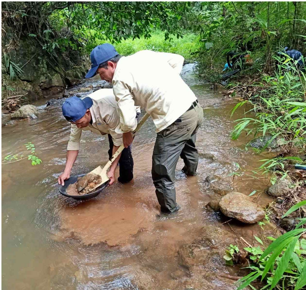
Figure 3. Sampling team at Tarlay panning concentrates from stream sediments.
