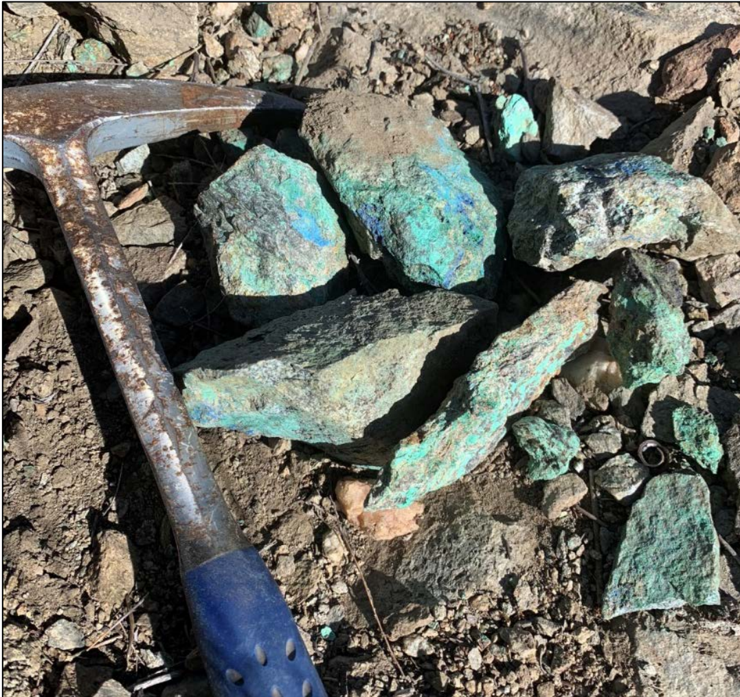
Figure 6: High-grade waste from dump material at OREX target assaying 9.15% Cu, 192 g/t Ag and 0.15 g/t Au. The sample was collected next to a small adit mined along a copper-bearing shear within the Leatherwood intrusive.
