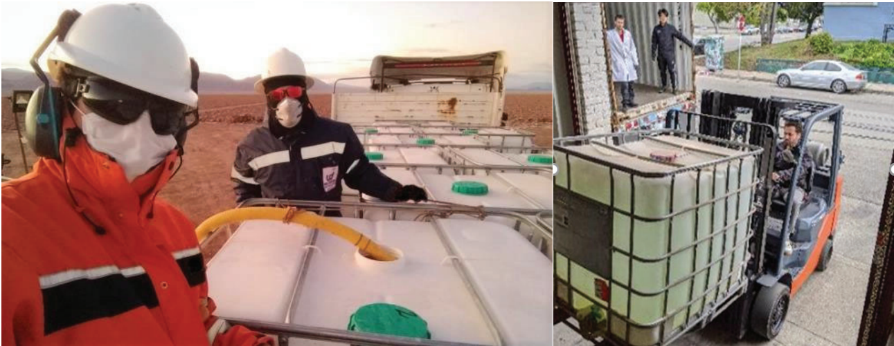
Figure 2: Lithium bearing brines being pumped into containers at the Kachi Lithium Brine Project. Containers delivered to Lilac's pilot plant module in Oakland, California
