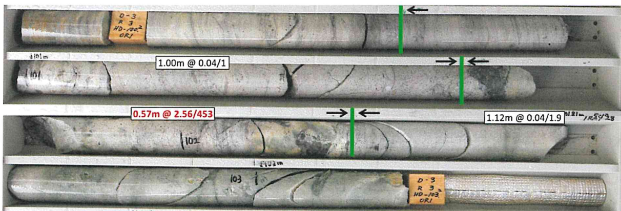
Photo 2 - DKDD008. Core photos with annotations such as 2.56/453 representing (g/t Au) / (g/t Ag).
