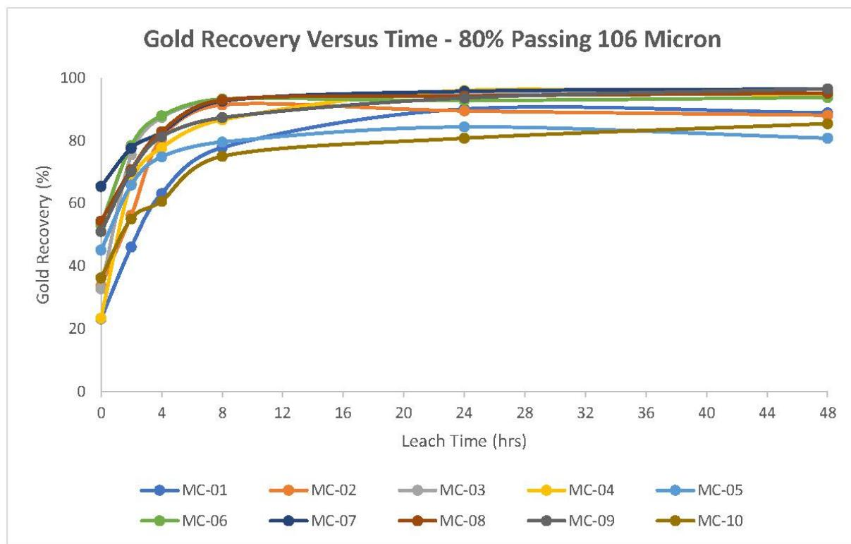
The kinetic leach curves show that most leaching is complete after 24 hours, with only samples MC09 and MC10 showing any significant leaching after that time.
