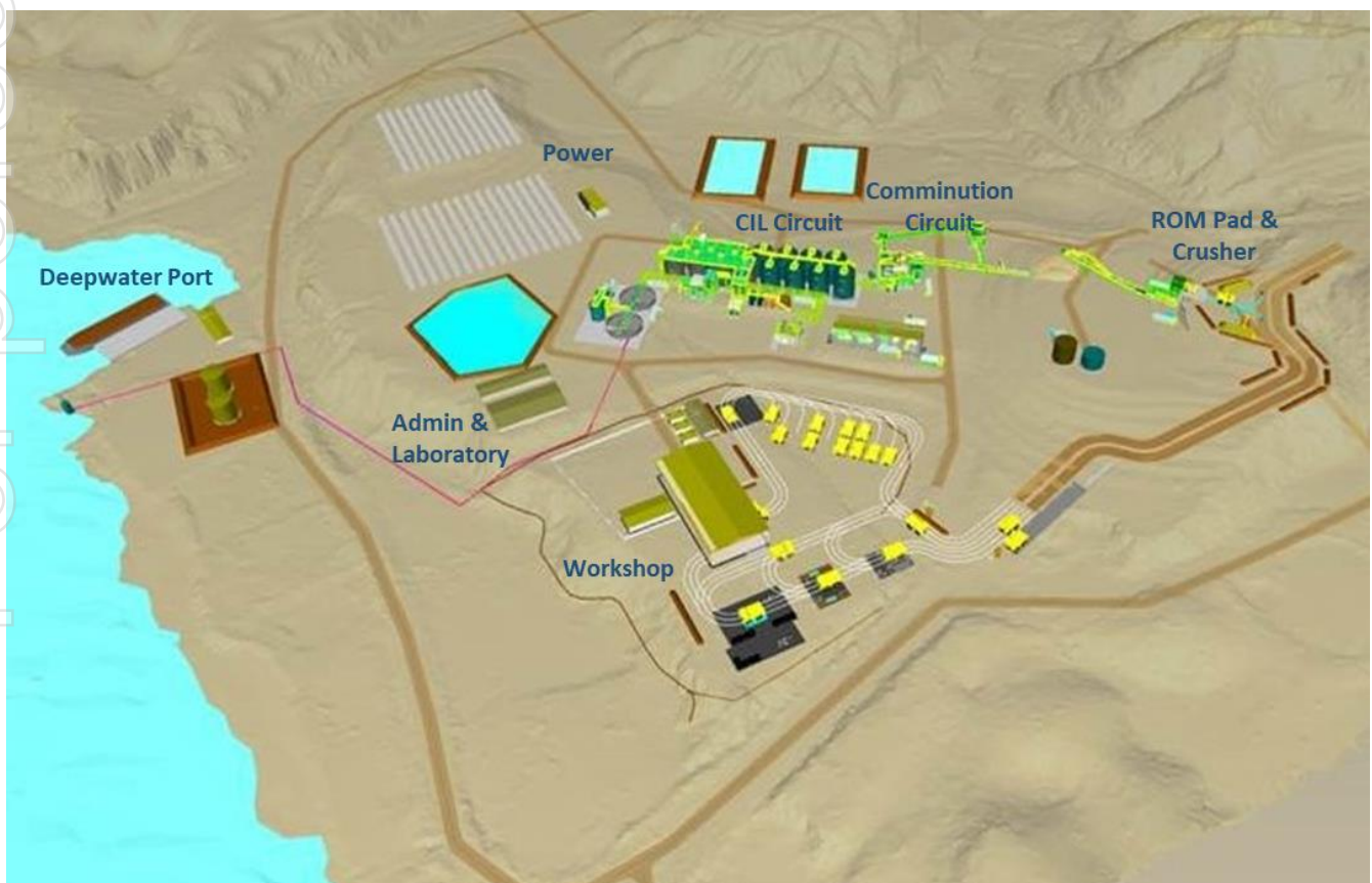
Figure 1. Preliminary process plant plans showing existing topography and located on the historical Placer mill site
