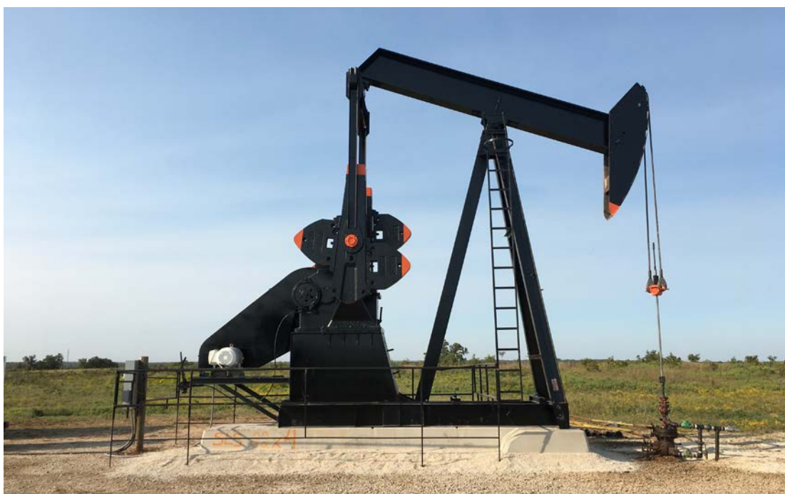
Figure 3. Pumping unit installed on the Mitchell Well in Carter County, Oklahoma
