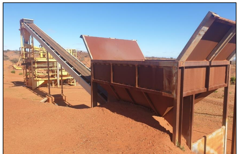
Figure 7. View from feed hopper along feed conveyor to wash-plant.
