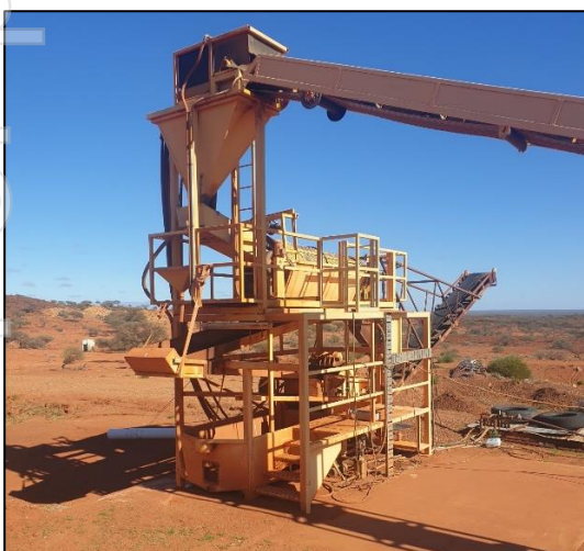
Figure 6. Fully operational 25-30tph “wash-plant” acquired as part of the acquisition.
