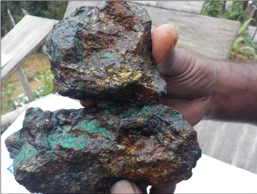
Figure 5. Sample number 152158, outcrop sample from Waa Creek, (assays 9.17% Cu and 1.03 g/t Au)
